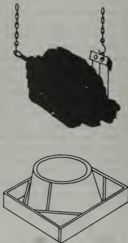
FIGURE 8-31. Hoisting engine for vertical packing.
